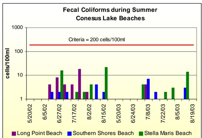
**Figure 4.** Plot shows count of fecal coliforms sampled in public beaches along Conesus Lake shore, May—August 2002 and 2003. Notice values are plotted using a logarithmic scale.
